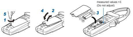
Do not adjust any screws other than the screw holding the battery cover in place. Do not adjust the three screws underneath the cover, which are used to adjust measured values, as doing so may prevent accurate measurement.
